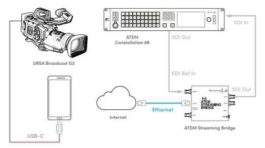
**NOTE** For streaming via an Ethernet adapter we recommend the Belkin USB-C to Gigabit Ethernet Adapter. While other USB-C to Ethernet adapters may work, the chipset used in the Belkin adapter is the most reliable for RTMP streaming video workflows.
