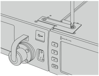
3 Turn the attached units back over and attach the rack ears to the outer edges near the front of both converters, using the supplied rack ear screws. Your converters are now ready to be installed into a rack using the mounting holes on both sides and standard rack screws.
