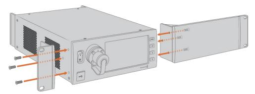
3 Use three of the supplied rack ear screws to attach a rack ear to the other side of your Studio Fiber Converter.
