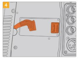
Plug the molex connector on Blackmagic Camera Fiber Converter into the molex power socket on your camera's rear panel.
