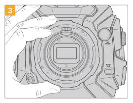
Carefully lift the lens mount away from the camera body. Keep the screws safely located close to the lens mount.
