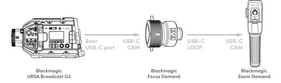
Daisy chaining allows for both units to be controlled using the rear USB-C port on your URSA Broadcast G2. For example, connect a USB-C cable into your camera's rear USB-C port and connect the other end of the cable into the focus demand's 'cam' port. With a second cable, plug the focus demand's 'loop' port into the zoom demand's 'cam' port.
