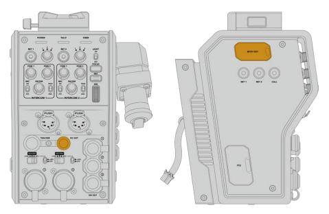
The DC out connector lets you power additional accessories, such as a monitor or external recording equipment
