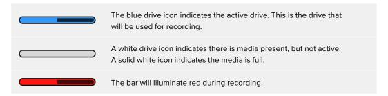
To switch recording to a different card or drive, press and hold the name or media bar of the card, USB-C flash disk or SSD that you wish to record to.
