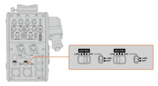
If you would like to connect microphones that aren't self powered, you can enable 48V phantom power. Move the phantom power switch to '+48V' to enable phantom power for any microphone connected to the XLR below, or 'off' to disable phantom power.
