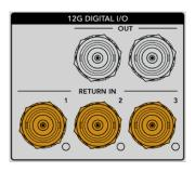
The return SDI inputs allow you to connect up to three return feeds from your switcher. These feeds will be fed to your camera so that they can be viewed by the camera operator, or fed out via SDI to other equipment.
