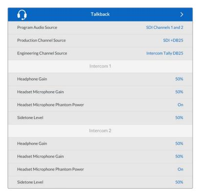
The intercom section will be grayed out when nothing is connected to the XLR inputs and will display 'connecting' during connection
