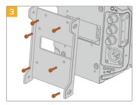
Attach Blackmagic Camera Fiber Converter's mounting bracket using 6 x 2.5mm Hex screws.
