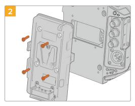
Unmount any battery plates currently fitted to your camera. For more information on mounting and unmounting battery plates, see the section 'mounting batteries' in this manual.
