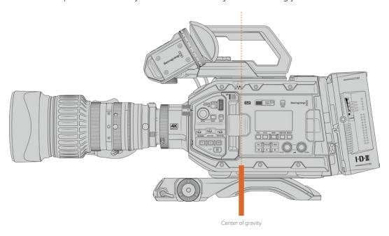
When mounting URSA Broadcast G2 on the URSA Mini shoulder pad, it's a good idea to mount the camera towards the rear of the shoulder pad base when using longer zoom lenses. This moves your camera rig's center of gravity back over the middle of the pad, making it easier to balance on your shoulder and rest steadily when sitting on a desk or flat surface. Refer to the 'URSA Mini Shoulder Kit' section later in this manual for more information on fitting the shoulder pad.
