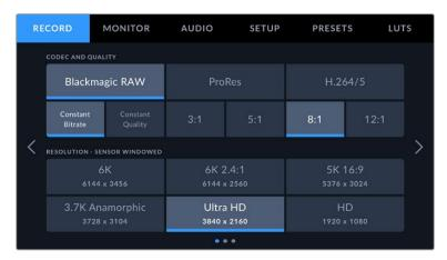
Tap the 'record,' 'monitor,' 'audio,' 'setup,' 'presets,' and 'LUTS' headings to move between your URSA Broadcast G2's dashboard tabs
