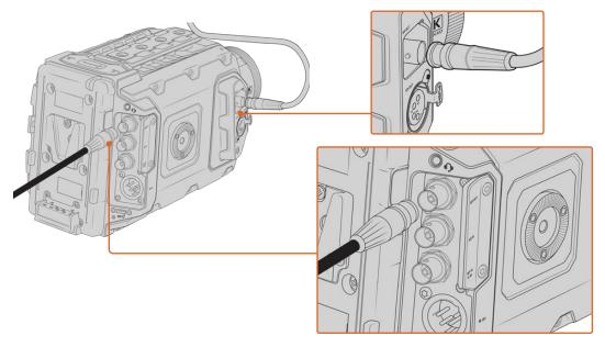
You can connect the 12G-SDI output to any 1080 HD or Ultra HD live production switcher or monitor. The HD monitoring output can be plugged into an external viewfinder, such as the Blackmagic URSA Viewfinder, or plugged into an external monitor when mounted to production equipment. For example a jib arm or crane
