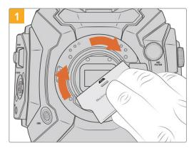
Gently insert the PL baffle into the center of the lens mount and turn until it is finger tight. Use the wide end of the baffle tool to tighten the baffle slightly. You need just enough pressure to keep it in place.
