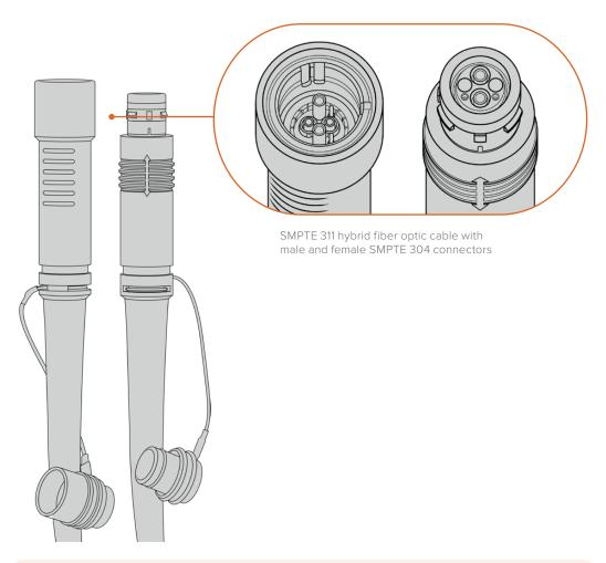
**NOTE** The male and female ends of a SMPTE 311 hybrid fiber optic cable can be identified by looking for the male and female pins inside the tip of the SMPTE 304 connector. The gender of the connectors is not determined by their outward appearance.
