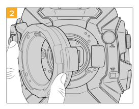
Ensure the pins on the PL mount for Cooke /i Technology are located at the 12 o'clock position.
