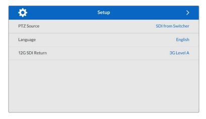
Select the source of PTZ commands using the PTZ source setting. You can select from 'SDI' or '9-pin', which correspond with the 'return in' SDI inputs and the DE-9 connector for PTZ on the rear of your Blackmagic Studio Fiber Converter.
