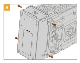
Attach URSA Mini Recorder to the mounting bracket using 2  $\times$  T10 torx screws on the left and right side of the brackets.
