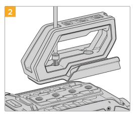
Fasten the handle to any two of your URSA Broadcast G2's top 1/4" mounting points using the two supplied 1/4" screws with a 3/16" Hex key driver. URSA Broadcast G2's rear two mounting points are recommended for most situations, but you can choose any pair for better weight balance when using large lenses.
