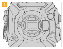
Place Blackmagic URSA Broadcast G2 vertically on a solid, clean bench top to ensure that the mount can be inserted vertically. If changing from the PL to the EF mount, ensure that you have removed the PL baffle before inserting the EF mount.
