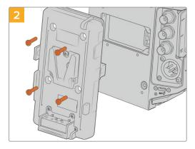
Remove the battery plate or molex power cover plate, if attached, using a phillips head screwdriver.
