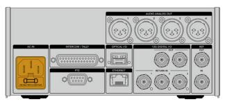
Connect power to your studio fiber converter via a standard IEC power cable
