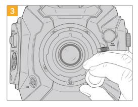
Loosely turn the five mounting screws until initial contact is made with the shoulder of the lens mount.
