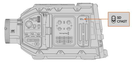
When recording to SD cards on URSA Broadcast G2 make sure the storage media selection switch is set to 'SD'
