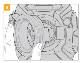
Place your lens mount onto the camera body, tighten screws and remount your lens and check if your lens focus marks are now in alignment with the focal distance. If not then continue steps 1 to 6, adjusting shimming a small amount at a time until your lens is hitting hits marks.
