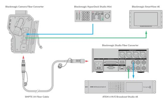
To confirm video, plug video sources into the return feed inputs on the studio unit, then view them on a monitor connected to the camera unit
