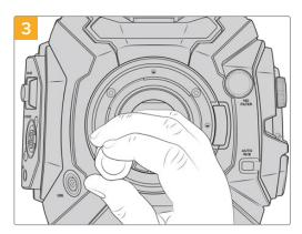
Loosely turn the four mounting screws until initial contact is made with the shoulder of the lens mount.
