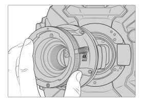
The B4 mount is removed by unscrewing the five M3 Hex screws and lifting the mount from the camera body.
