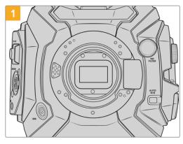
Place Blackmagic URSA Broadcast G2 vertically on a solid, clean bench top to ensure the mount can be attached vertically. If changing from the PL to the F mount, ensure that you have removed the PL baffle before inserting the F mount.
