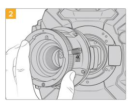
Keeping the original .50mm shim in place, gently put the Blackmagic URSA Broadcast G2 B4 mount onto the camera body ensuring the red dot is at the 12 o'clock position.
