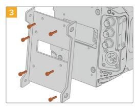
Attach URSA Mini Recorder's mounting bracket using  $6 \times T10$  torx screws.
