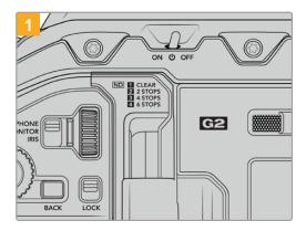
Power off URSA Broadcast G2 by moving the 'power' switch to 'off'.
