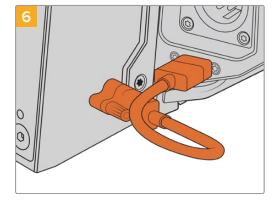
Connect the Mini Recorder's USB-C cable to the USB-C data port on the rear of URSA Broadcast G2. Tighten the locking connectors with your fingers, or use a 2mm hex key driver.
