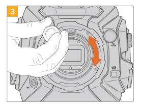
Loosely turn the five mounting screws until initial contact is made with the shoulder of the lens mount. To access all five screws, you will need to rotate the PL locking ring, as some holes are obscured when the ring is either open or closed.
