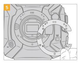
Add or remove shims to slightly change the depth of your mount. It is a good idea to start with a small shim thickness such as a 0.10mm.
