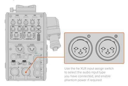
The camera audio is embedded into channels 1 and 2 of the camera feed, and the 2 audio inputs on the back of the camera fiber converter are embedded as channels 3 and 4. All 4 audio channels are also deembedded at the other end on the studio fiber converter as analog audio outputs.
