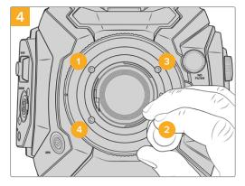
Using the 2mm Hex driver, or torque wrench with 2mm Hex key, apply one full turn of pressure to mounting screw 1, followed by one full turn to screw 2, and repeat for screw 3 and then 4. Continue to apply one full turn to each screw in the sequence above until all screws have reached the maximum torque of 0.45Nm.
