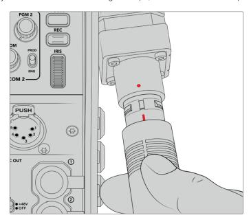
Align the red indicators to connect the SMPTE Hybrid Fiber Optic cable to the large connector on the Blackmagic Camera Fiber Converter
