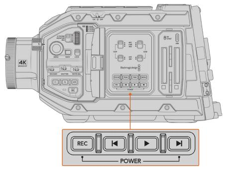
If you need to, you can also hold down the record and forward skip buttons on the control panel behind the LCD to power your camera on or off
