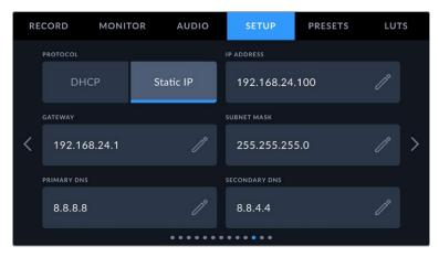
You can connect to a network using a DHCP or a static IP address
