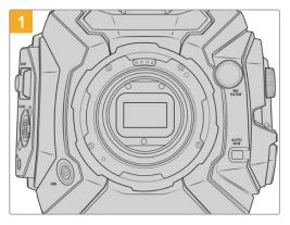
Place URSA Broadcast G2 vertically on a solid, clean bench top and remove your lens or dust cap. The filter covering the sensor will be exposed for the duration of the shimming process, so it's important to keep the filter as clean as possible. Be careful not to touch the filter while shimming mounts.
