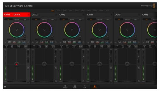
Try adjusting the iris and pedestal in ATEM Software Control's camera page to test camera control
