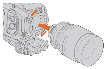
Attaching and removing a PL lens
