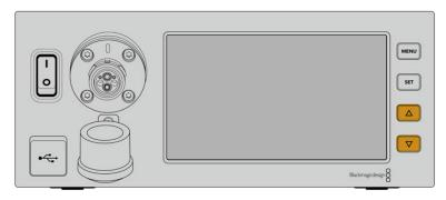
Press the up and down arrow buttons to scroll through the four possible sources and to navigate through the menu
