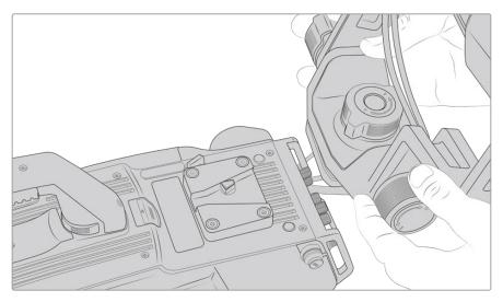
V-Lock mount plate being attached to 3rd party camera
