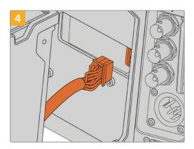
Plug the molex connector on URSA Mini Recorder into the molex socket on your camera's rear panel.
