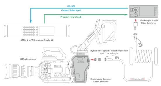
The Blackmagic camera and studio fiber converters connect via optical fiber to provide efficient SDI video, power, talkback, tally and control signals via a single SMPTE fiber optic cable.
