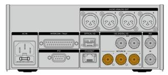
Plug the program return feed from the switcher and other return sources into the 'return' inputs on the studio unit's rear panel
