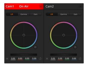
Each camera controller displays the channel status so you know which camera is on air. Use the color wheels to adjust each YRGB channel's lift, gamma and gain settings
