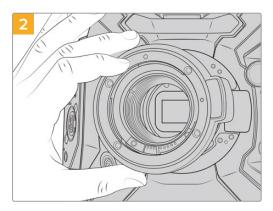
Carefully place the Blackmagic URSA Mini Pro EF mount onto the camera body ensuring the red dot is at the 12 o'clock position.
