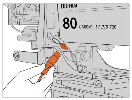
Add additional power to your box lens by plugging in a 4 pin XLR cable
