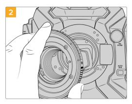
Carefully place the Blackmagic URSA Mini Pro F mount onto the camera body ensuring the white dot is at the 2 o'clock position.
