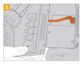
Slide the Blackmagic Camera Fiber Converter onto the mounting bracket, and attach it using 2 x 2.5mm Hex screws on each side of the bracket.
