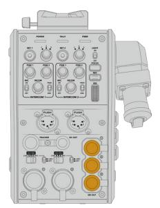
The three return feed loop outputs can be connected to SDI equipment near the camera, for example a teleprompter or monitor
