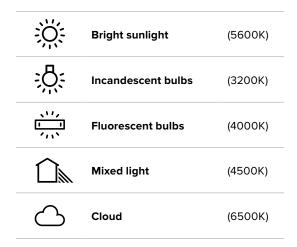
You can customize any of these presets by tapping or holding the arrow icons to the left and right of the temperature indicator in the bottom left of the 'white balance' menu. Each tap moves the color temperature up or down 50K, but holding the arrow icons down will increase these increments for faster changes. Alternatively, you can move the temperature slider in the middle of the 'white balance' menu.
