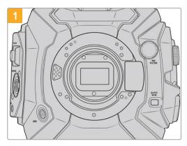
Place Blackmagic URSA Broadcast G2 vertically on a solid, clean bench top to ensure that the mount can be inserted vertically.
