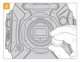
Remove the screws holding your mount in place using a 2.0mm Hex driver. For more information on removing particular mounts, see the 'interchangeable lens mount' section in this manual.
