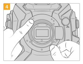
Note the alignment of the existing shim with the alignment pin at the 11 o'clock position.
