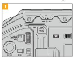
Ensure your camera is powered off. If using URSA Broadcast G2 or URSA Mini Pro, power it off by moving the power switch to 'off'.
