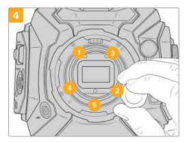
Using the 2mm Hex driver, or torque wrench with 2mm Hex key, apply one full turn of pressure to mounting screw 1, followed by one full turn to screw 2. Repeat for screws 3 and 4, then 5. Continue to apply one full turn to each screw in the sequence above until all screws have reached the maximum torque of 0.45Nm.
